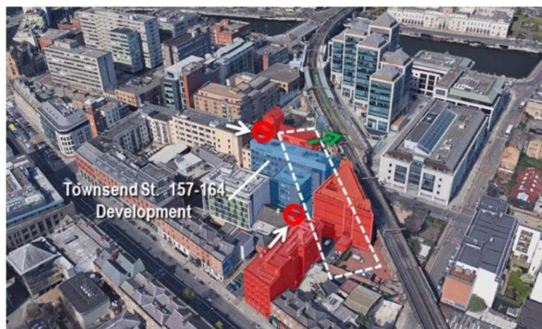
Option 3: Location moved southwards under Townsend Street (Open box with top-down construction)
